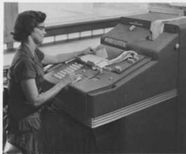
▲ Chris Letzeisen shown operating an electro-mechanical bank proof machine during a customer demonstration.
