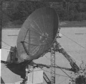
◀ A close-up view of the 36-foot diameter microwave antenna used in satellite/computer transmission experiments.
