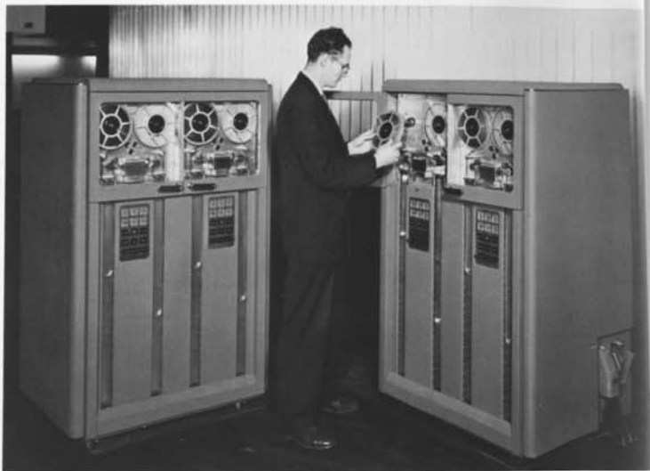
▲ A demonstration of tape reel removal. The vacuum columns clearly show the long tape stress during reel reversal.
