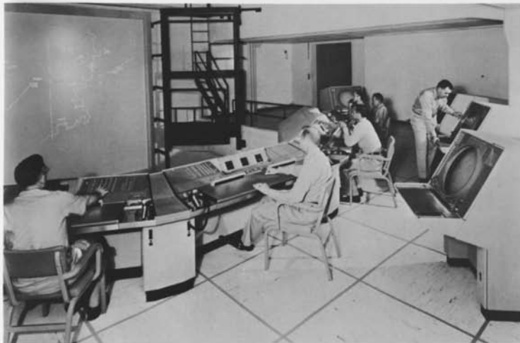
▲ SAGE was one of the first large computer networks to provide man-machine interaction in "real time" as events were occurring. This system,
