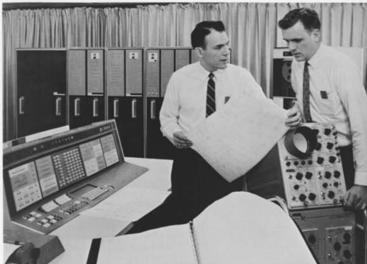
▲ Circuit designs for the new IBM 7080 data processing system were prepared by the new system's predecessor, the IBM 705 III. Here, during test, the circuitry is checked by
